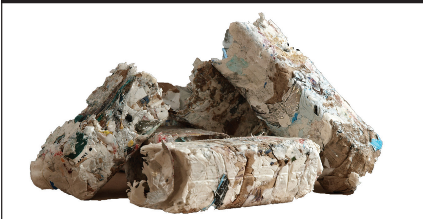
The finished fuel – Enviro Fuel Cubes® – ready for delivery to the customer
